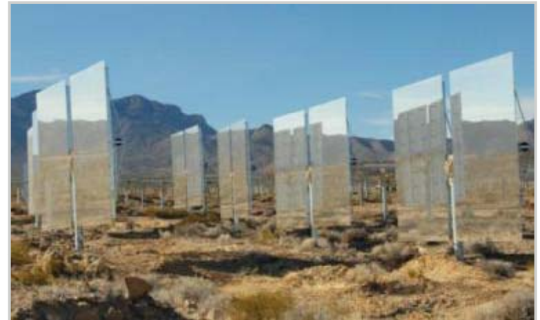
Two flat glass mirrors (2.3m x 3.3m) mounted on a single pylon equipped with a computer-controlled drive system
