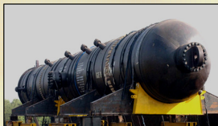
665 MT HGCO reactor for Valero St. Charles refinery in the US by G&B
